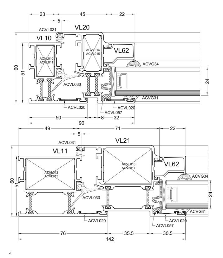
system (depth 51mm) for windows and doors with thermal break
